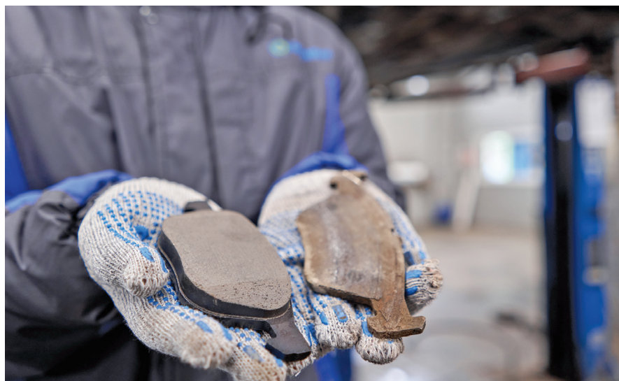
EXTRA PADDING – A mechanic shows the difference between a new brake pad and one that has been worn thin. Image: malkovkosta. Adobe Stock.
